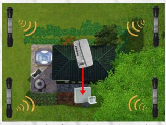
Roboguard interfaces easily to most alarm panels
